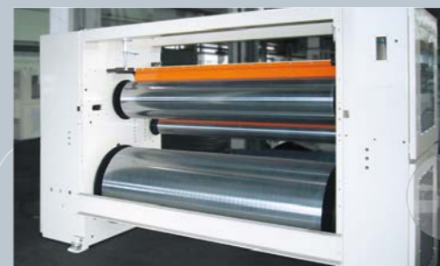
Cooling roller rack at Vits in Langenfeld, Germany, equipped with three cooling rollers (ø 200 mm, ø 400 mm and ø 800 mm) from AR Walzen
